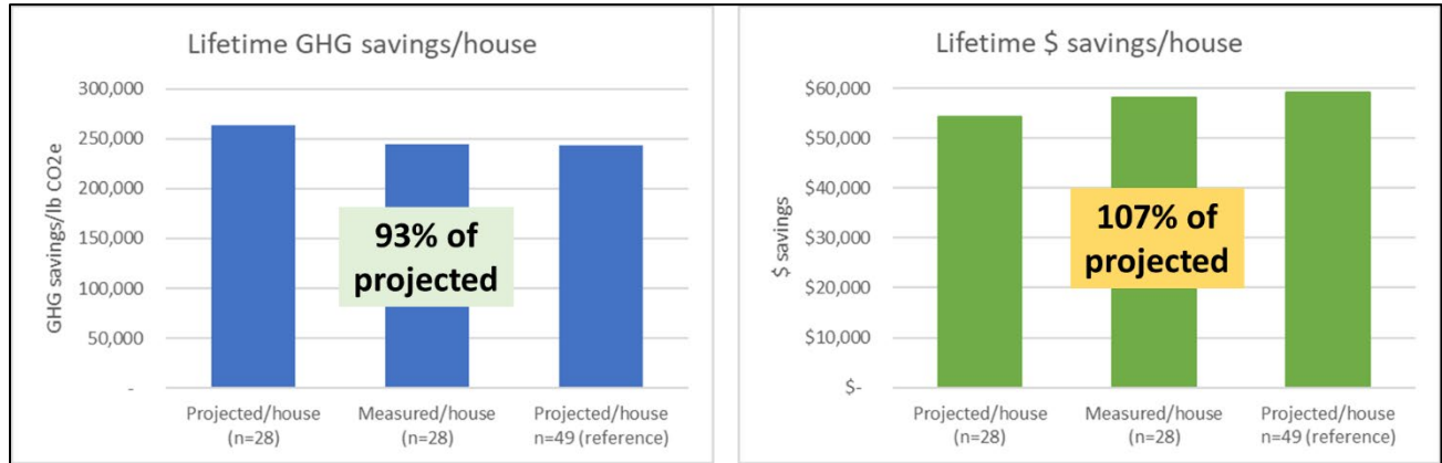
Figure 16. Measured and projected lifetime emissions and cost savings per home.
