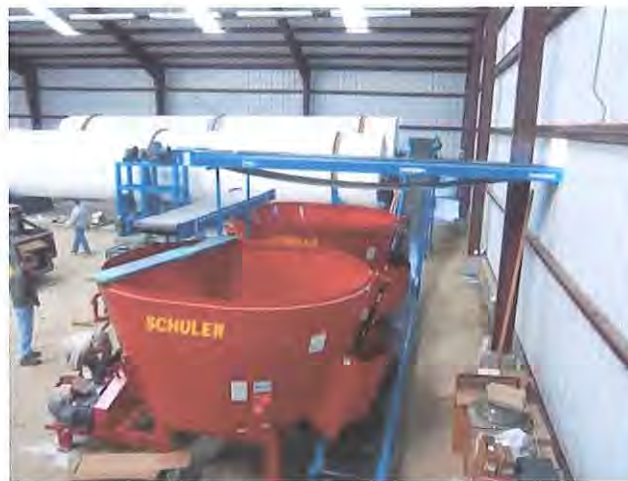
Figure 15: Twin mixer/feed systems with BW 1050 drums in pole barn process 30 TPD
