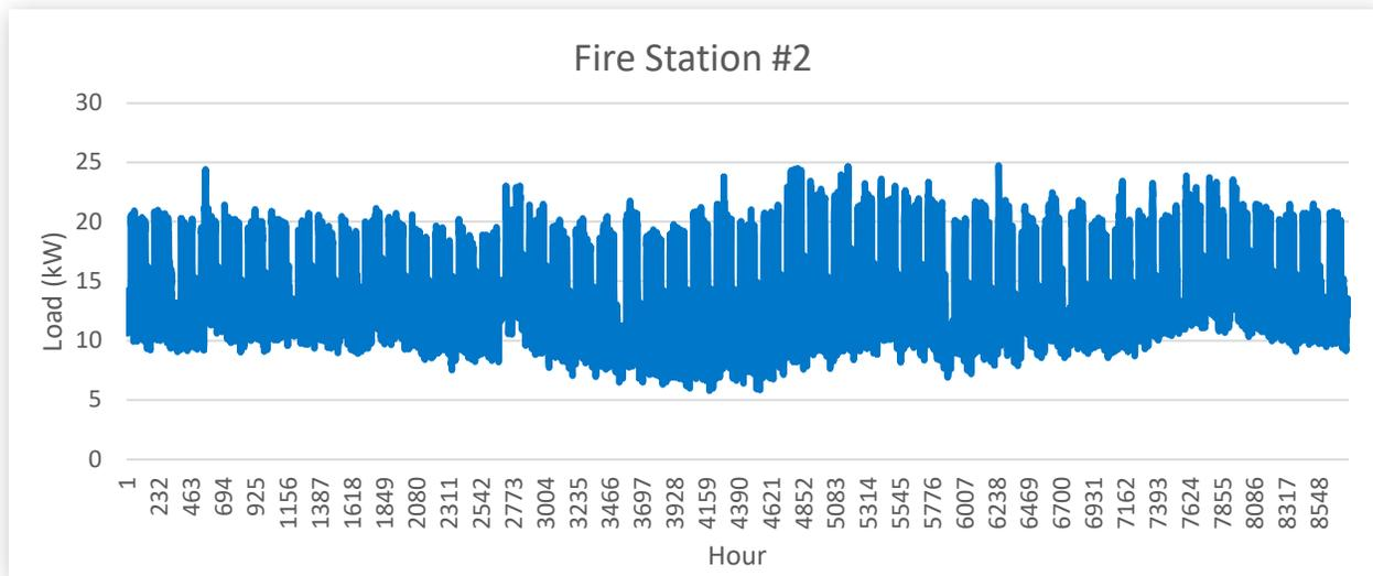
Figure 22. FS2 Estimated Hourly Electricity Load Profile in Peak Load Day
