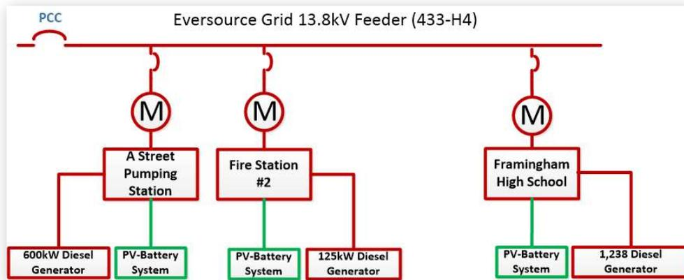
All the stakeholders are connected to the same 13.8kV feeder, which reduces the community microgrid islanding and interconnection complexity.
