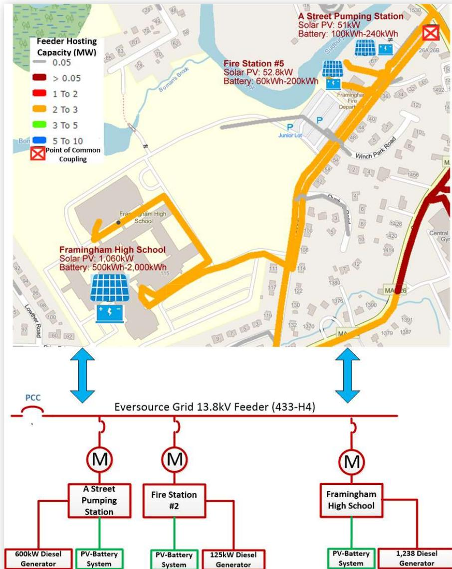
As shown in Figure 1, all the stakeholder locations are fed by the 13.8kV feeder. This configuration served to reduce the complexity of community microgrid islanding and interconnection.
