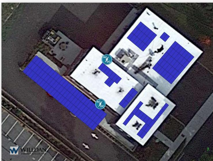
Figure 29. PS Solar PV Layout (51.2 kW)
