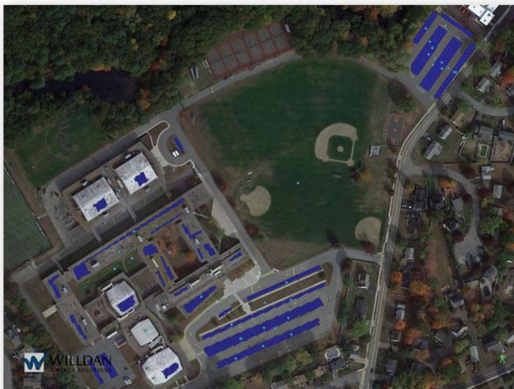
Figure 28. FS Solar PV Layout (52.8 kW)
